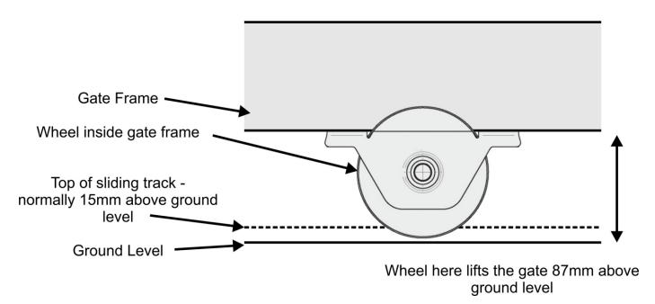
If using standard bolt down track the height of the track is 15mm. If using concrete in track you should leave 15mm above ground level.
